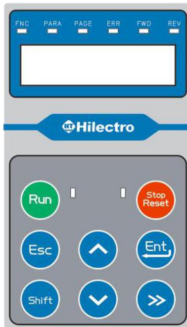
Figure 5.1 Digital operation panel
